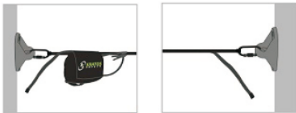
Case 1: There are anchorage points available (EN 795 Type A)
